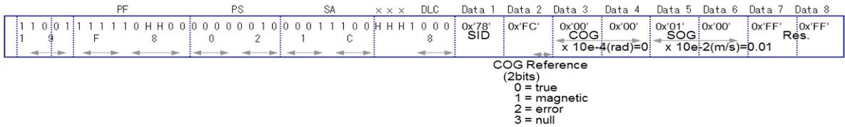
2. PGN : 129029 (0x'01F805'), Priority:3, Data length:8(DLC=0x'8')x8, Data bytes =下図参照
