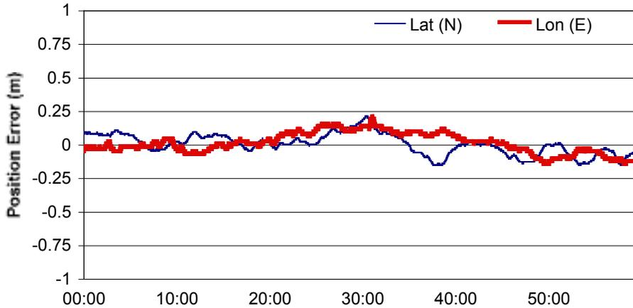
**Figure 6: Position Error using WAAS (24 hours total)**
